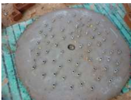
Figure 31: Filtration bed of iron removal plant
